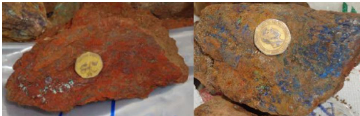
Figure 24: Typical Cu Ore at Ibagá; SEDEX and VMS respectively (Photo courtesy by Kalimenze)
